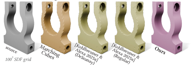
Fig. 4. Competing SDF reconstruction methods that rely on marching cubes or tetrahedra exhibit artifacts near sharp features, except when those features happen to align closely with the underlying elements of the volumetric mesh or grid. Our method exhibits no such bias.
